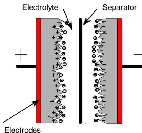
Figure 2: Supercapacitor sketch
