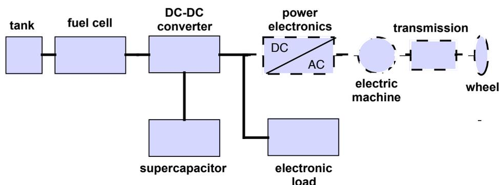
Figure 2: Schematic view of the power train system combining a fuel cell and supercapacitors. For the tests presented in this paper an electronic load replaced the motor.
