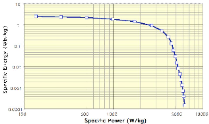
Figure 4: Ragone Plot of the 800-F capacitor with PSI electrodes.
