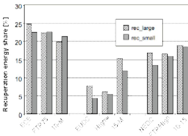
Figure 1: Potential energy savings by recuperation in a small vehicle (mass 750 kg, rolling resistance 0.01, air drag 0.6 m<sup>2</sup>) and in a large vehicle (mass 1500 kg, rolling resistance 0.013, air drag 0.7 m<sup>2</sup>) in different driving cycles.
