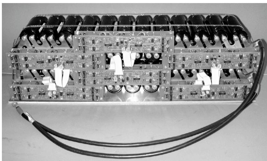
Figure 5: The supercapacitor module developed jointly by PSI and montena, combined with a voltage-balancing (charge-exchange) unit developed at EPFL. Its key data: 48 cells, 60 V, 60 F, ESR=20 m $\Omega$ ., max. energy 30 Wh, max. power 45 kW.
