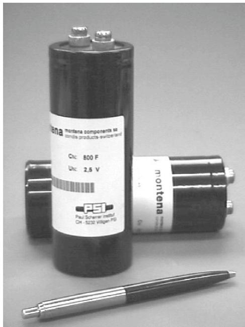
Figure 3. Supercapacitor cells with a capacitance of 800 F developed in a collaboration between PSI and montena SA.
