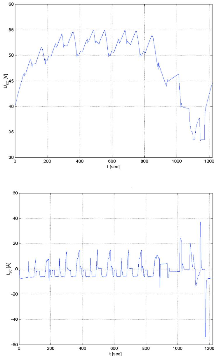
Figure 7: Voltage of the supercapacitor module (top) and the current flowing into and out of the module (bottom) in a reduced NEDC ( $P_{EM} + 1000$ ). At the end of the cycle the charge level of the module is higher than at the start.
