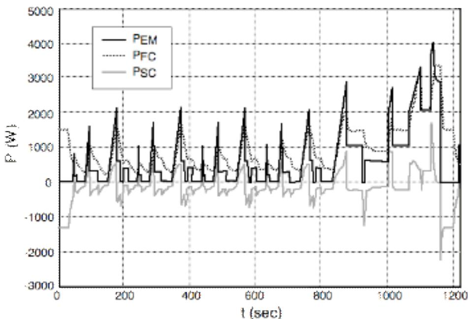
Figure 6: Power demand and measured power of the electric motor, the supercapacitor, and the fuel cell system during a NEDC.
