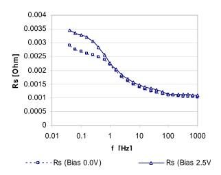
Figure 4: Series resistance frequency spectrum of a BCAP0350
