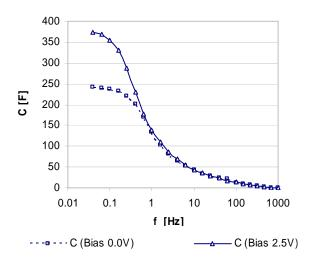
Figure 3: Capacitance frequency spectrum of a BCAP0350
