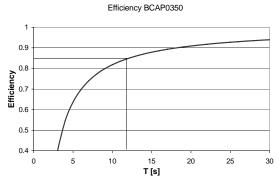
Figure 6: BCAP0350 discharge efficiency
