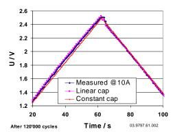
Figure 2: 10 A charging curve for the BOOSTCAP® type BCAP0350 with a nominal capacitance of 350F and a series resistance of 2.4  $m\Omega$ , measured after 120'000 cycles.
