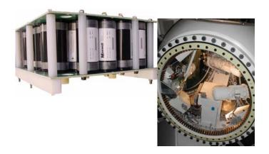
Figure 9: Rotor hub with independent electro-mechanical pitch propulsion units and emergency power pack containing 34 large cells rated at 2'700 F, a nominal capacitance of 78 F and a nominal voltage of 76 VDC
