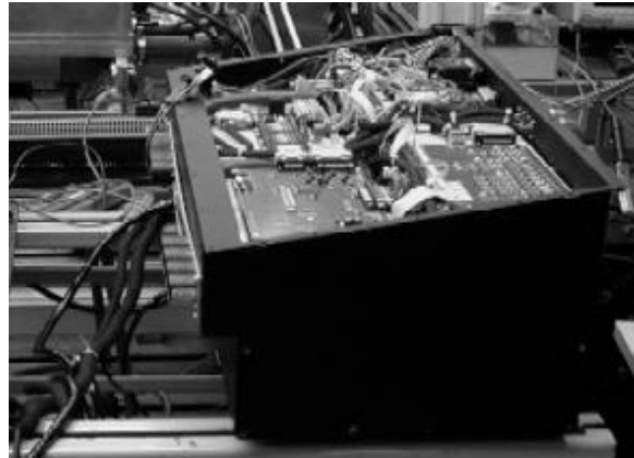
Figure 13: The fully assembled BOOSTCAP ® module in its storage box
