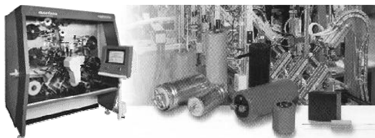
Figure 3: Montena winding machine and assembly line
