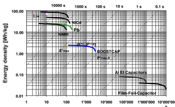
Figure 1: The Power density [W/kg] Ragone plot shows the energy density vs. the power density
