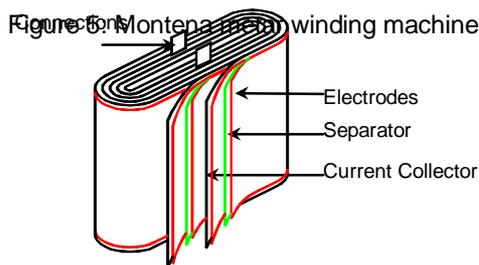
Figure 4: Supercapacitor flat winding
