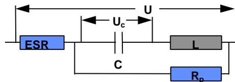
Figure 6: Supercapacitor equivalent circuit
