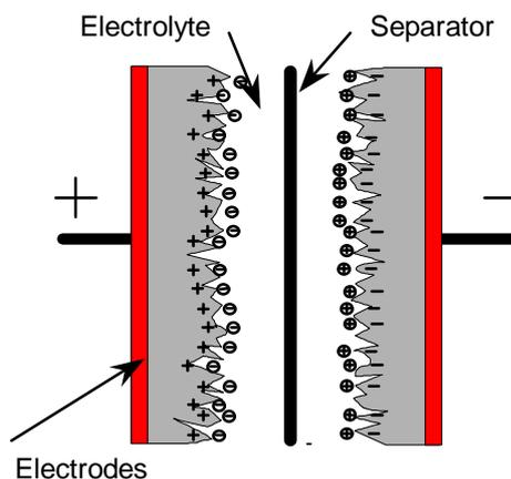
Figure 2: Supercapacitor sketch
